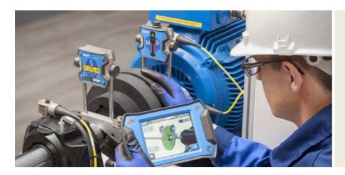
Shaft alignment is recommended for almost every industry, as it enables machine uptime to be significantly improved and maintenance costs to be reduced. The simplicity of the TKSA 41 provides greater confidence for the performance of alignment tasks on all types of horizontal rotating machines.
