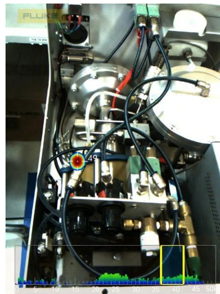
Air tightness inspection of complicated equipment pipelines
